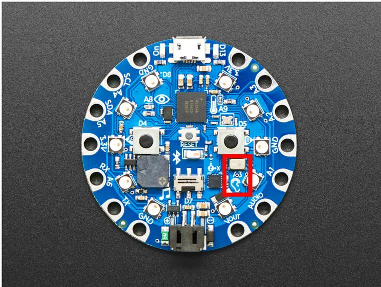
This example turns the LEDs red each time you make a loud sound. Try clapping or blowing onto the microphone to trigger it.
